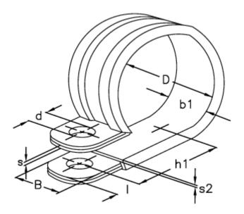
$\begin{array}{lll} \text{b1} & = 31.0 \\ \text{d} & = 10.5 \\ \text{Diameter D} = 49 \\ \text{h1} & = 42.0 \\ \text{I} & = 10.0 \\ \text{s} & = 1.00 \\ \text{s2} & = 3.0 \\ \text{Width B} & = 25 \\ \end{array}$
